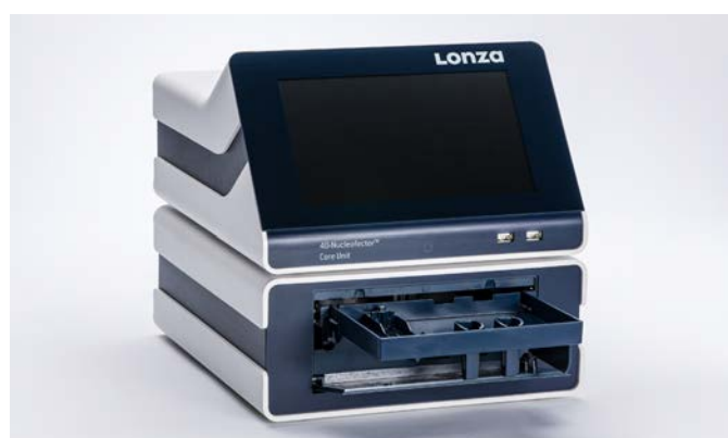
Figure 3.2: Exemplary appearance of the tray after rescuing the sample and before 4D-Nucleofector System can be turned on again.
