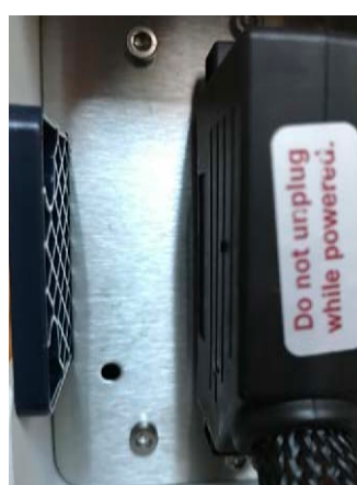
Figure 2.8: (A/B) Opening for hexagon screw driver on the back of 4D-Nucleofector® System.
