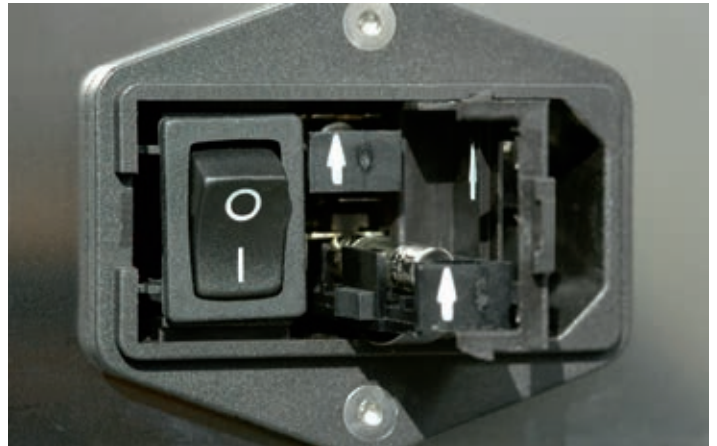
Figure 2.0: Opened fuse receptacles
